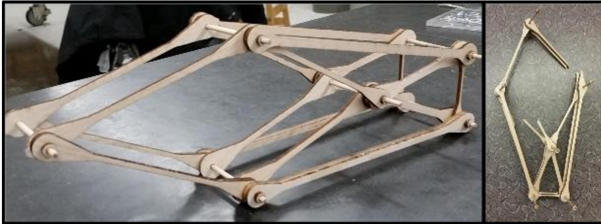
Figure 17. The third truss design before and after testing
