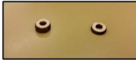
Figure 14. Difference between balsa wood densities in the caps when squeezed with full strength
