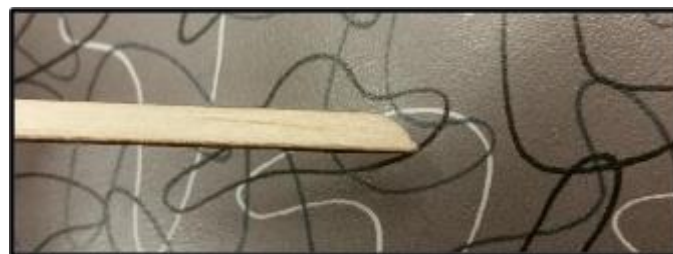
Figure 18. The broken member with characteristic 45 degree angle seen in torsional failure
