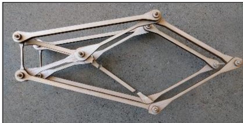
Figure 21. The final design after breaking. The broken member is displayed to illustrate break location.
