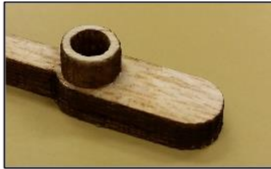
Figure 12. An idea to account for bearing stress. Further iterations proved this design decision unnecessary
